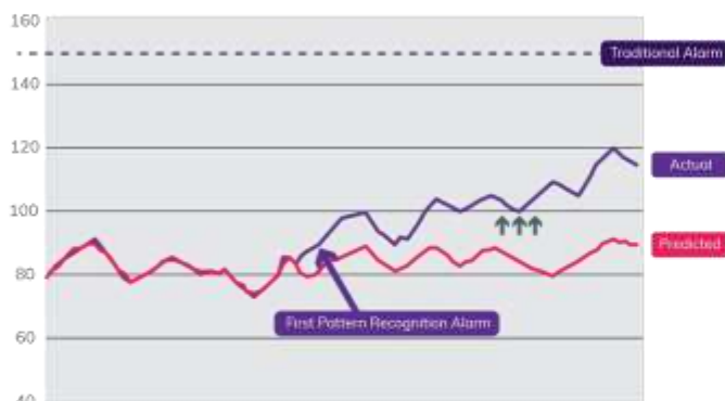
Predictive Asset Analytics makes it easy to identify anomalies and provides notification of abnormal conditions before operational alarms.
